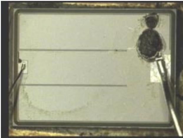
Figure 6. 20 A, 500 V MOSFET Avalanche Failure.
